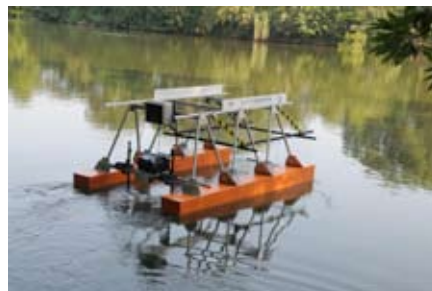
The Carlton J. Kell High School Robotics Team's Trash Collecting Robot for rivers, lakes, and streams.
